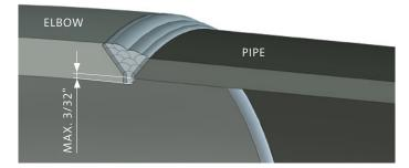
Figure 2: Minimum misalignment < <u>3/32</u>" (<u>2.38</u> mm) using Erne Fittings high-precision segmentable elbows enabling pipe line production without back welding operations.
